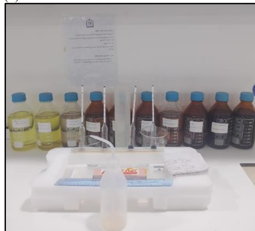
Figure2: The Sp.gr test of gasoline, kerosene, gas oil, and lubricating oils
